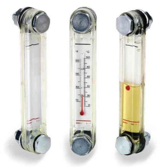
Thermoplastic level gauges made from transparent polyamide which provides good mechanical resistance and is impervious to mineral oil, gasoline, lubricants, petroleum, solvents and most chemical agents (please refer to technnical table N.1 page 58); avoid contact with alcohol based solutions and antifreeze liquids at high temperatures and hot water over 80°C
