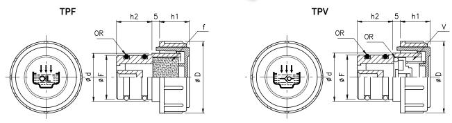
f = Air filter V = One-way check valve OR = O-Ring NBR seal
