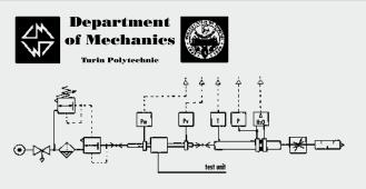
• Flow tests carried out at the Department of Mechanics, Turin Polytechnic, using the computerized test bench following CETOP RP50R recommendations (ISO DIS 6358-2-approved) with ISO 5167 diaphragm gauge.
