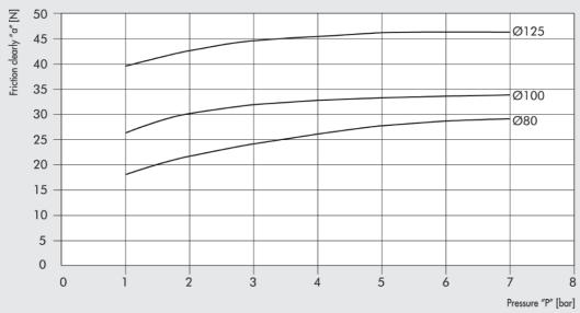
The clean friction values "a" in N have been obtained by inserting in the back chamber the pressure "P" in bars, and simultaneously by detecting the necessary force "F" in N to make the rod re-enter, applying the following formula:
